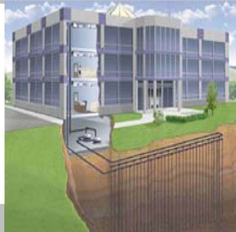
Ground source condenser water from closed loop type ground source geothermal wells.
