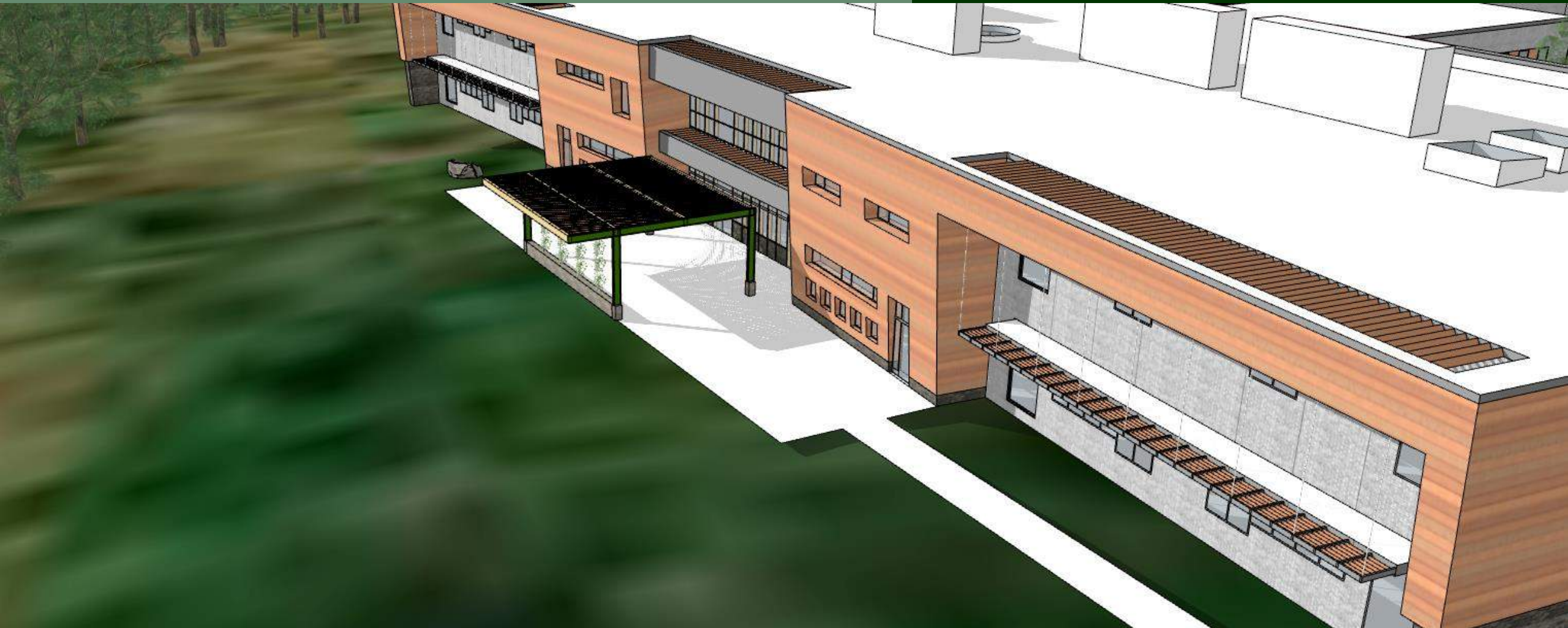
View of integrated shading on southern elevation
