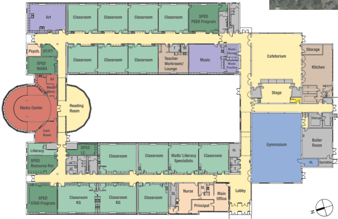
< Exhibit 2.13 Downey Elementary School First Floor Plan
